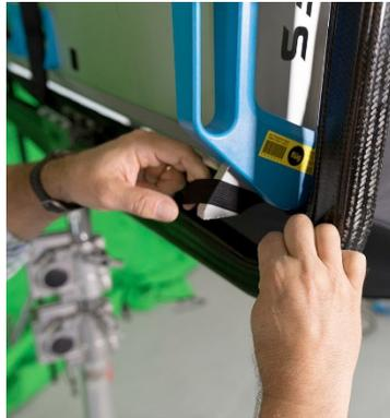
3. Using the supplied straps, secure the Lightbank to the fixture. One set of straps will run vertically across the back of the fixture. The other set will run horizontally. Secure the straps using the attached D Rings. Again, ensure that the side marked "This Way Up" is pointing up.
