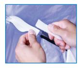
With the Lightbank on the fixture, attach the internal baffle to the white hook and loop tabs on the inside of the Lightbank.
