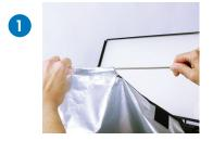
Insert Poles into sleeves. Keep the pole sleeve straight as you slide each pole through the sleeve to the end of each corner.
